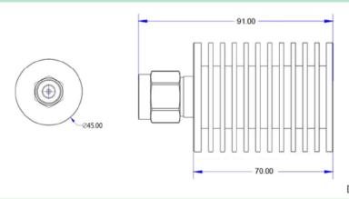
Unit:mm Dimension tolerance:±2%
